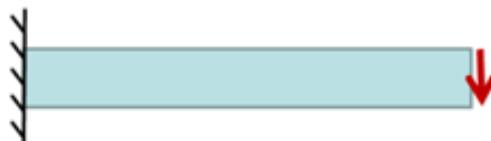
A new model is presented in this paper, dealing with timber beams subjected to transversal loads. For simplicity only in-plane displacements will be considered. Two different kinds of buckling modes (orthogonal eigenmodes) of great importance can appear and both should be checked in order to determine the loadbearing capacity.
