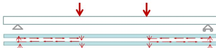
When the E-modulus is constant over the cross section the total loadbearing capacity is three times that of one individual beam part. This assumption of a constant stiffness over the cross section will often result in misleading results. A much better strength prediction is normally obtained if the radial variation of the longitudinal E-modulus from pith to bark is considered.
