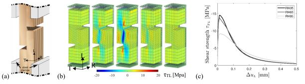
Figure 1: Shear test of adhesive-wood joints (glutin-based glue and European beech): (a) experimental setup; (b) shear stress (τ<sub>TL</sub>) propagation (from left to right): initial (u<sub>L</sub>=0 mm), elastic, peak before failure (u<sub>L</sub>=0.196 mm), directly after failure, final condition (u<sub>L</sub>=0.5 mm); (c) dependency of the shear stress on moisture [MC<sub>beech</sub>(RH): 6.8%(35%), 12.1%(65%), 23.8%(95%)] [2]
