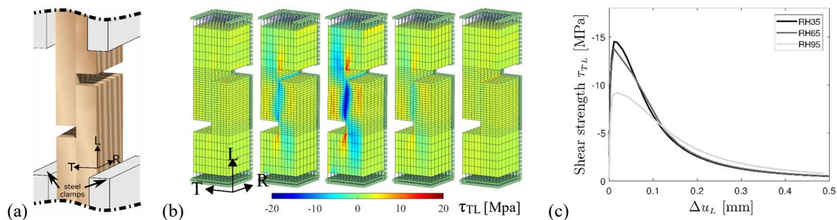
Figure 1: Shear test of adhesive-wood joints (gluten-based glue and European beech): (a) experimental setup; (b) shear stress ( $\tau_{TL}$ ) propagation (from left to right): initial ( $u_L=0$  mm), elastic, peak before failure ( $u_L=0.196$  mm), directly after failure, final condition ( $u_L=0.5$  mm); (c) dependency of the shear stress on moisture [MC<sub>beech</sub>(RH): 6.8%(35%), 12.1%(65%), 23.8%(95%)] [2]
