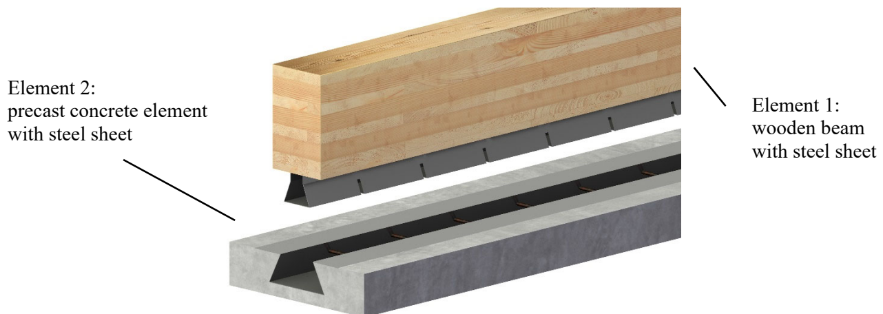
Figure 1: Schematic Sketch of the New Timber-Concrete Composite Construction
