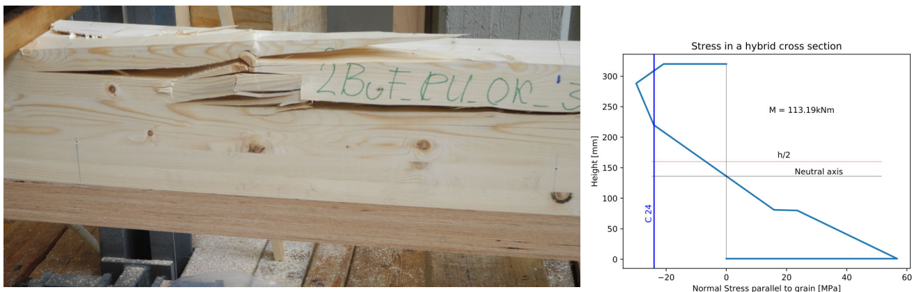
Figure 1: GLT beam with 25 % Beech LVL Reinforcement
