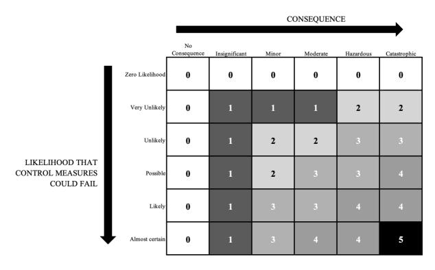
Figure 2 Example Error Sensitivity Matrix
