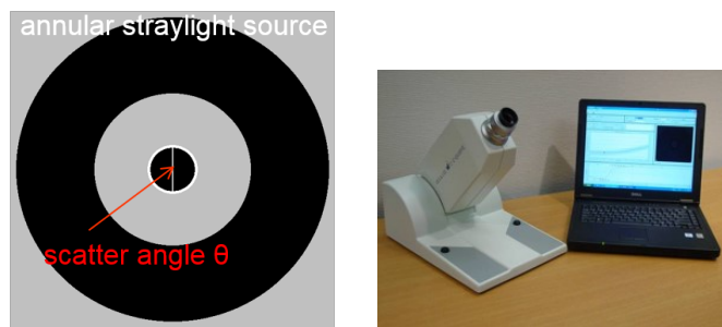
Figure 3: Left: test field as presented by the C-Quant (right). The measurement involves a bipartite field surrounded by an annulus. Flickering light is presented within the annulus. Light from the annulus is scattered towards the bipartite field and its intensity is measured using the psychophysical CC method (van den Berg et al., 2005). The annulus has inner radius of 5° and outer radius of 10°, which makes for an effective mean radius of 7° (van den Berg, 1995). Please see text for details on the CC method.
